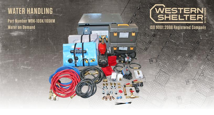
Designed to support most water handling applications in the field, the WA-WDK10 supports up to 10 people with a 4 WSD shower system. Complete with hot, cold and gray water delivery hoses, the kit will support 8 shower heads and one 3-basin sink. Each kit includes a 500 gallon potable bladder and a 500 gallon gray water bladder as well as sump pump kits and a primary water distribution pump.
