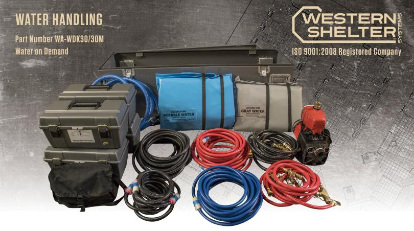
Designed to support most water handling applications in the field, the WA-WDK30 supports up to 30 people with a 4 WSD shower system. Complete with hot, cold and gray water delivery hoses, the kit will support 8 shower heads and one 3-basin sink. Each kit includes a 500 gallon potable bladder and a 500 gallon gray water bladder as well as sump pump kits and a primary water distribution pump.
